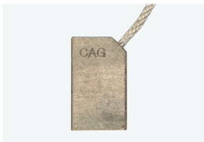
PART NO. H102032 Material: CAG, Model: 601 Dimensions: 20x10x32 mm Flexible: FS 4 mm 2 -80 mm Terminal SRO-6
